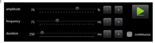
This group allows you to tune the hopper actuator and the duration of the vibration.
