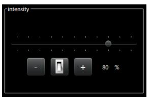
The light intensity group contains controls to adjust intensity of backlight.
