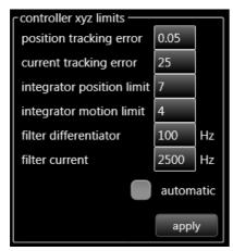
The fields for this zone make it possible to adjust the controller limits parameters.
