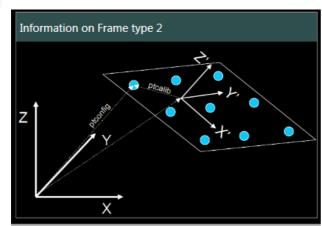
An explanatory drawing makes it possible to view which type of frame has been used.
