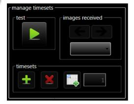
This group allows you to manage the timesets. A timeset is a set of parameters which allows you to acquire an image. Thereby, if several images are needed, add a new timeset.
