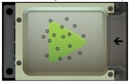
• If the sequence has a "centering" vibration defined, nine buttons are displayed. They give information to the sequence about the position of the parts on the plate and allow you to test the sequence with various part arrangements.
