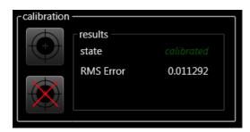
The group gives access to the calibration execution and to the result of the calibration.
