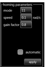
The fields for this zone make it possible to adjust the homing mode, speed and gain factor parameters.
