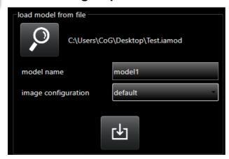
This group contains few controls which allow to load a model recipe with a specific model name and a selected image configuration name.
