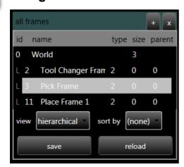
This zone is used to view all of the frames created, as well as any possible parent.
