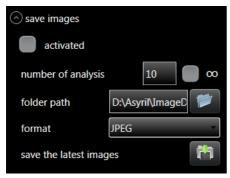
The activated checkbox allows you to switch on/off the saving of images with the parameters below. The saving is done at the end of analysis.
