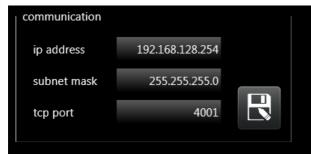
In this group, you can change IP address, subnet mask and topport of Asycube electronic. Click on the button to apply the modifications.
