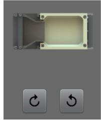
Choose the orientation in which to display the Asycube view in the Hmi (not applicable on all pages).
