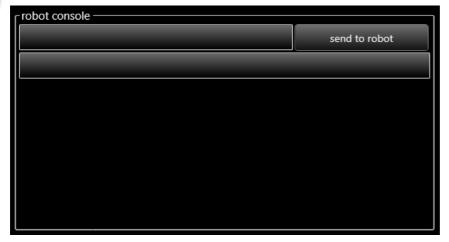
The console is used to send a TCP command directly to the robot from the text zone. The response sent by the robot is transcribed in the bottom area.
