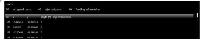
This group displays the list of the good parts found and/or the rejected parts depending of the selection in the results selection group.
