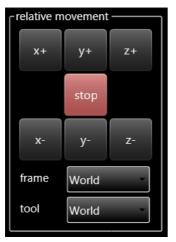
The buttons in this zone are used to move the robot relative to the current position in a given frame and using a specified tool.
