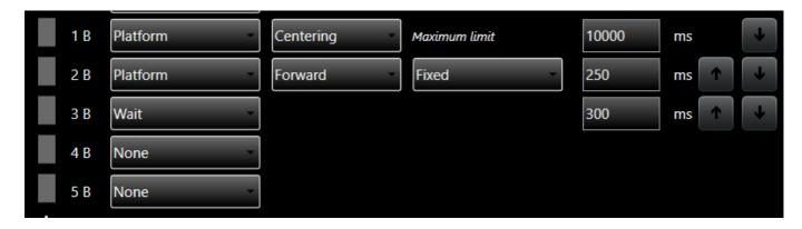
You can use the arrows on the left to switch command lines up or down within the same block (no switching between A and B blocks are allowed).
