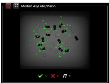
This zone is one of all the available displays. Each camera has its own display and the images are displayed together with the number of parts accepted, refused, and the number of parts detected by the feeding information tool.
