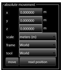
The buttons in this zone are used to move the robot to an absolute position in a given frame and using a specified tool.
