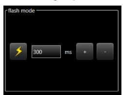
The flash mode group contains controls to adjust flash duration of backlight.
