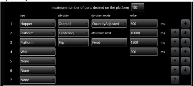
This group allows you to tune the selected sequence. The sequence is composed of 7 actions. Each action can be a platform vibration, a hopper vibration, a waiting time or a purge action if that option is enabled (requires a specific platform). Depending of the type of action, some parameters have to be chosen:
