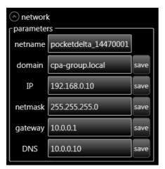
This area is used to modify the domain name, or IP address of the robot.
