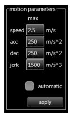
The fields for this zone make it possible to adjust the motion speed, acceleration, deceleration and jerk parameters.
