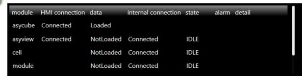
This table provides more information about the connection state of each module (robot, process, asycube and asyview) and indicates whether an alarm has occurred. In addition, the "data" column indicates whether the data related to each module has been loaded or not.
