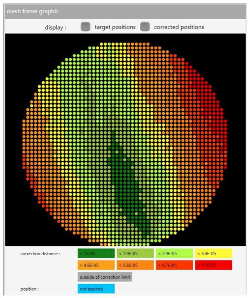
This area is used to display a graph of the results obtained during the calibration of this frame. The colours represent the correction distance between the setpoint position and the position given by the robot.
