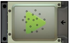
• If the sequence has an action defined with the vibration centering, nine buttons are displayed. They give informations to the sequence about the position of the parts on the plate and allow to test the sequence with many parts arrangement.
