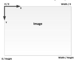
Width = number of pixels / line Height = number of pixels / column The camera 0,0 position is always at the top left of this representation.
