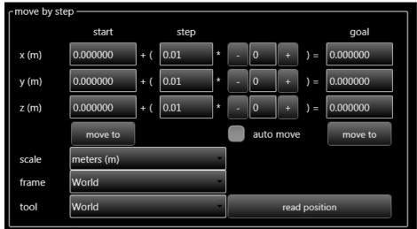
The buttons in this zone make it possible to move the robot in a step by step manner. The size of the step and the starting setpoint must be specified.
