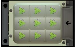
• The number of parts on platform is useful when using a vibration with a duration mode "Quantity Adjusted" because the Asycube will change the duration of the vibration depending of the number of the parts on the platform. As with the nine buttons, it is useful to test the sequence with a large number of parts on the platform.
