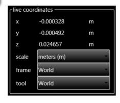
This field indicates the position of the robot in real time. By default, the position is sent in the basic reference (world: frame 0 tool 0, in meters). The dropdown lists make it possible to select which frame and which tool should be used to read the current position of the robot.
