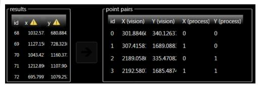
This group allows you to select 4 positions in the list of positions measured by the camera and to place it in the corresponding points pair.
