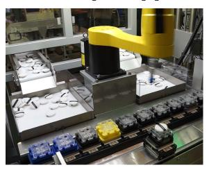
The camera looking on the Asycube detects precisely the parts with the right side facing up and gives the angular orientation information to the robot for a fast and delicate pick and place.
